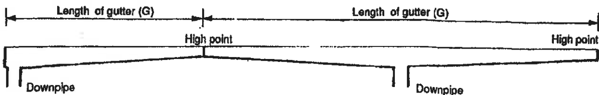
FIGURE 2.2 MEASURING GUTTER LENGTH
