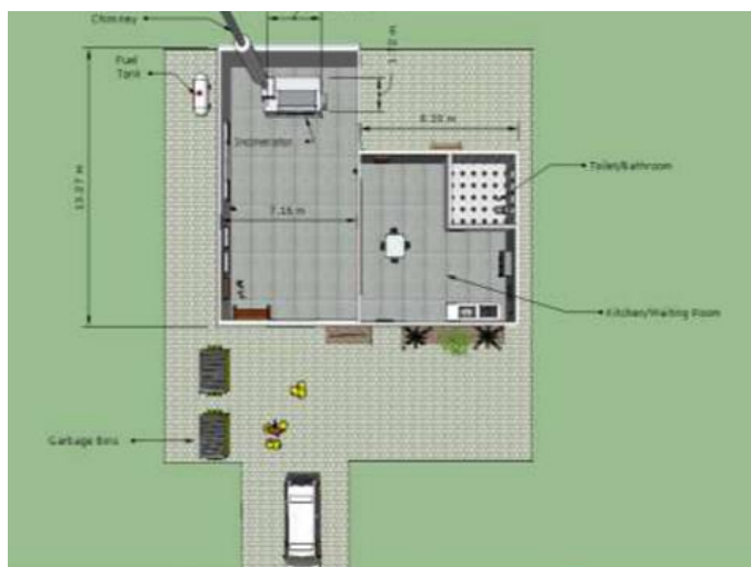
Figure 2: Site layout of the Naboro Incinerator (LionGIS, 2022)
